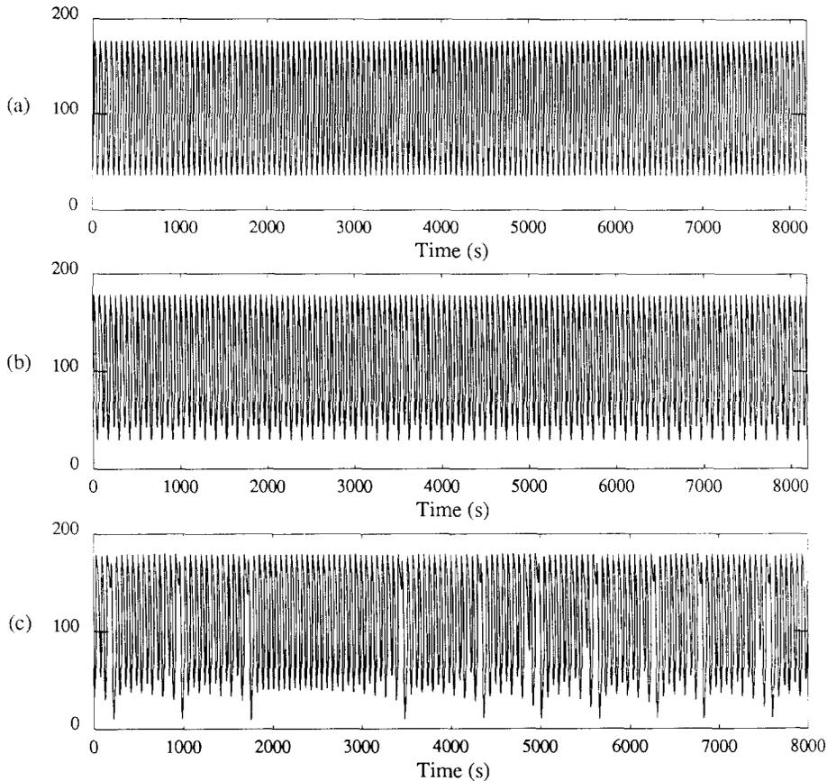
Fig. 5. Time series in bromide ion potential for a supercritical period doubling bifurcation. (a) A period-one limit cycle at  $\epsilon = -2.4 \times 10^{-3}$  is followed by (b) a period-two cycle at  $\epsilon = +6.6 \times 10^{-3}$  whose subharmonic amplitude is observed to grow continuously from zero with increasing  $\epsilon$ . (c) At  $\epsilon = +2.85 \times 10^{-2}$  an intermittent type of dynamics exists with reinjections directly onto the unstable 1-cycle.
