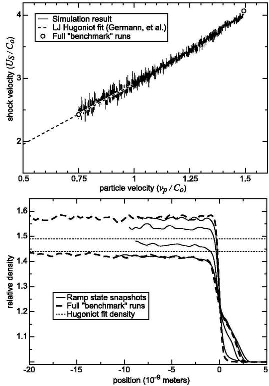
**FIGURE 2.** (top) Results of the Continuous Hugoniot Method, the fit of Germann et al. [1], and bookend benchmark runs. (bottom) Density profiles snapshots from a shock strength ramp (solid), from the initial and terminal benchmarks (dashed), and from the Hugoniot fit (dotted).
