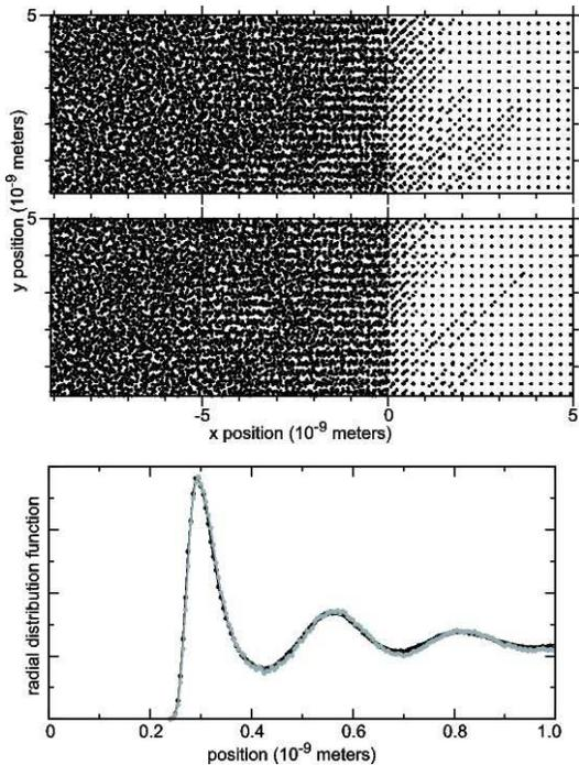
**FIGURE 3. Structural dynamics and rdf comparison** – Particle slices in the region of the shock front for states from (middle) the Continuous Hugoniot Method and (top) the terminal benchmark. Also shown (bottom) is a comparison of radial distribution functions for the compressed material extending 10 nm behind each front.  $v_p = 1.5 C_o$ .
