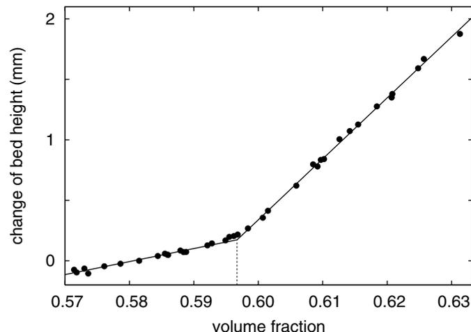
Fig. 4: Change in the height of the bed relative to the original bed height for a rod inserted to a depth of 60 mm. The transition occurs at  $\phi = 0.597$ . The bed is slightly deformed near the rod but not sufficiently to change its average height.
