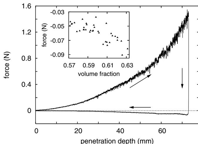
Fig. 3: Forces measured during a full cycle of insertion and withdrawal at a volume fraction  $\phi = 0.602$ . The speed of the rod is 10 mm/min in both directions. The inset shows the withdrawal force measured at a depth of 70 mm for the same experiments as in fig. 2.
