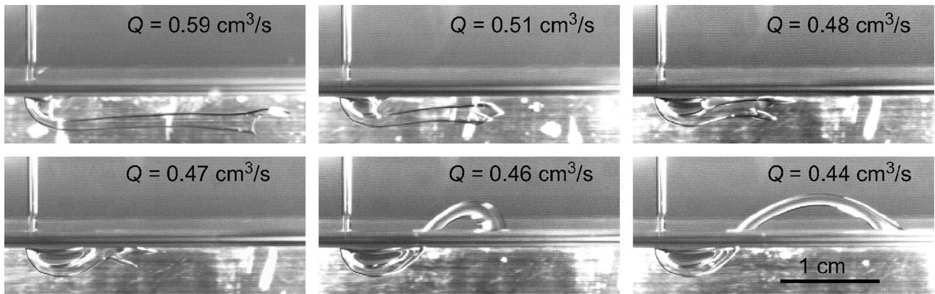
FIG. 1. Jet bouncing spontaneously as the flow rate  $Q$  rapidly decreases. Conditions:  $\mu=361$  mPa s,  $H=4.2$  cm, and  $V_{\text{bath}}=5.2$  cm/s. The relative times of each image are 0, 0.46, 0.66, 0.71, 0.82, and 0.90 s. The white splotches below the surface are bright reflections from the aluminum background (figure enhanced online).
