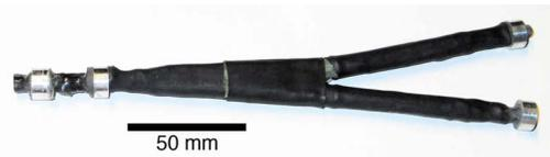
FIG. 4. (Color online) Photograph of completed split fiber bundle. The bundle is 8 in. in length and the two back ends are split about 2 in.
