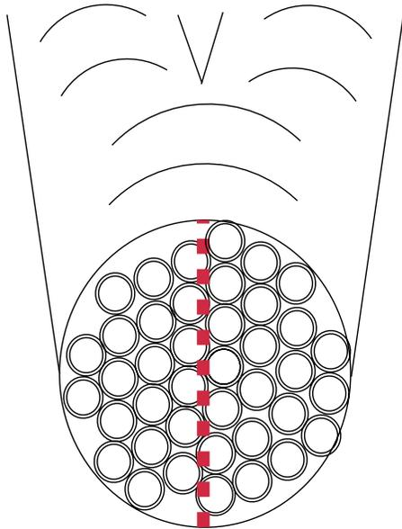
FIG. 2. (Color online) Schematic of the front end of the fiber optic waveguide splitter. Fibers on the left side of the red dashed line were sorted into one bundle on the back end while fibers on the right side were sorted on the other end. A laser and knife edge was used to split the waveguide into two nearly equal parts.
