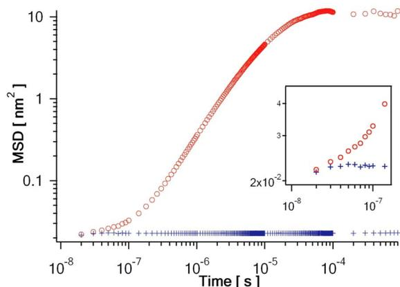
FIG. 5. (Color online) Mean square displacement of a 1  $\mu\text{m}$  polystyrene bead in an optical trap (red circles) with the noise background shown (blue crosses). The temporal resolution of the detector is around 30 ns with spatial resolution of about 1  $\text{\AA}$ .
