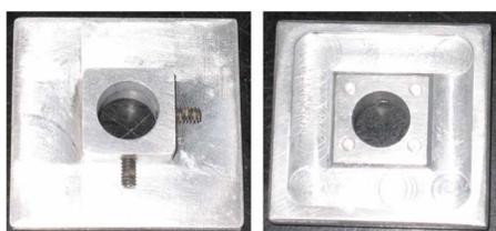
FIG. 3. (Color online) Photographs of the top (left) and bottom (right) view of the aluminum holder. The aluminum rings on the fiber bundle fit tightly into the holder. The set screws lock the bundle in place for polishing.
