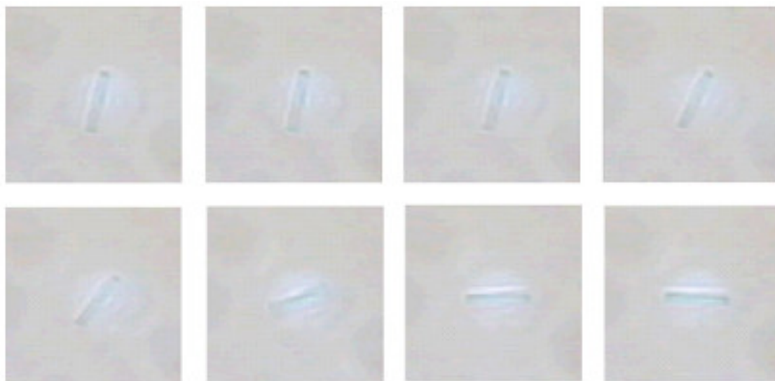
Figure 3. Microscopic glass cylinders following the rotating plane of polarization of the trapping beam. The length of the cylinder is 1.8 \mu\text{m} . Source: Bishop et al. (2003).
