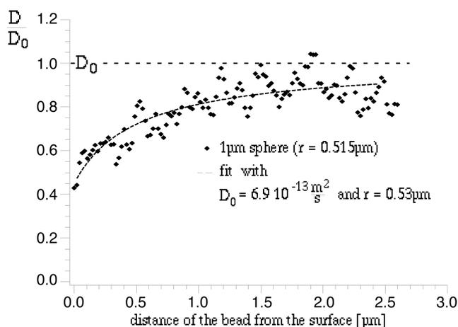
**Fig. 4.** Local viscosity measurement. Decrease of the diffusion coefficient of a sphere approaching a surface measured for a polystyrene sphere with  $r=515\text{nm}$  using the PFM. The dotted line shows the theoretical prediction by Happel and Brenner fitted for  $r=530\text{nm}$  and a free solution diffusion constant of  $D=6.9 \cdot 10^{-13}\text{m}^2/\text{s}$ .
