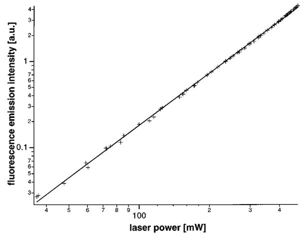
FIG. 2. Emission intensity recorded as a function of the excitation light intensity. The experiment was performed after a fluorescently labeled latex bead with a diameter of 1.03 μm had been captured by the optical tweezers. The excitation power in the focal plane was estimated to be 480 mW.
