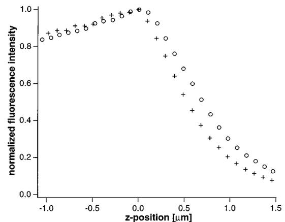
FIG. 3. The fluorescence emission of a bead captured by optical tweezers and monitored as a function of the relative axial position to the cover glass surface. Negative values indicate a position above the specimen (i.e., in solution). (+++) The probe approaches the cover slip. (○○○) The probe approaches the soft biological material in neurons on the same cover slip.
