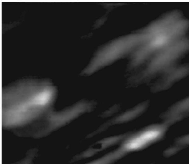
FIG. 5. Near-field optical image of a gold-coated nuclear filter having the mean pore size of 500 nm. A HeNe laser was used to image (the gold layer thickness was 30 nm, and the scan size was  $7 \times 6 \mu\text{m}^2$ ).
