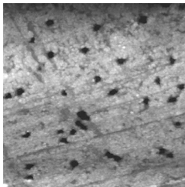
FIG. 4. Tapping-mode AFM image of a nuclear filter having holes with mean size of 25 nm (scan size:  $1 \times 1 \mu\text{m}^2$ ).
