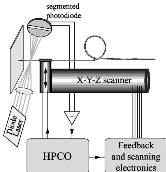
FIG. 3. Schematic diagram of the optical scheme for shear-force distance regulation. The signal from the segmented photodiode, due to the laser light scattered by the dithering fiber, is used as input to the HPCO, which in turn drives the piezotube to maintain oscillating the fiber at its resonance frequency.
