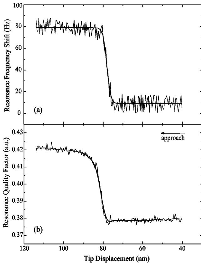
FIG. 8. Approach curves of the fiber tip to a glass slide surface recorded in the nonoptical shear-force detection scheme. (a) The resonance frequency and (b) quality factor were recorded simultaneously, and both increase upon contact.
