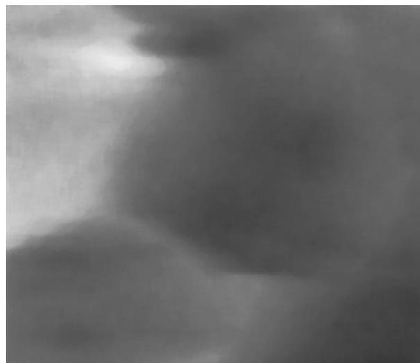
FIG. 7. Quality factor image of a gold-coated polymer film recorded with the optical scheme-based HPCO. “Grains” of different elastic properties are probably imperfections in the metal coating (scan size:  $6.7 \times 5.7 \mu\text{m}^2$ ).
