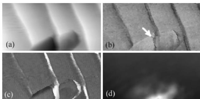
FIG. 6. A  $2.6 \times 5.5 \mu\text{m}^2$  scan of a CD-ROM surface using the nonoptical HPCO-controlled shear-force scheme for distance regulation. (a) Topography; (b) quality factor; (c) resonance frequency; (d) near-field optical image.
