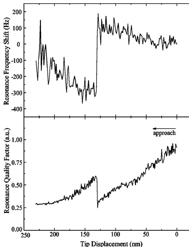
FIG. 10. Resonance frequency and quality factor during the approach of the fiber tip to a glass slide surface, recorded simultaneously with the optical shear-force detection scheme. It shows a probable transition between two regimes of tip-sample interaction.
