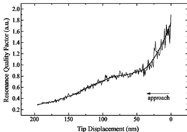
FIG. 9. Quality factor  $Q$  during the approach of the fiber tip to a glass slide recorded using the optical shear-force detection scheme. It shows the effect of the large oscillation amplitude.
