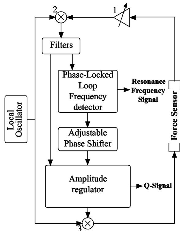
FIG. 2. Schematic diagram of the heterodyne phase-controlled oscillator. 1—input amplifier, 2—input mixer, 3—single sideband output mixer.
