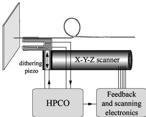
FIG. 1. Schematic diagram of the shear-force distance regulation scheme based on a tuning fork (nonoptical detection). The HPCO maintains driving the fiber glued to the tuning fork at its resonance frequency as it interacts with the sample. The signal generated on the piezoelectrical tuning fork serves as input to the HPCO.
