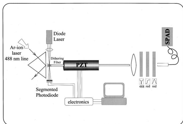
FIG. 2. Schematic of the SNOM-based FRET experiment. The 488 nm spectral line of a cw argon ion laser has been focused onto the glass prism surface in the conditions of total internal reflection (spot diameter  $\sim 300 \mu\text{m}$  and laser irradiation intensity  $I$  was  $15 \text{ W/cm}^2$ ). SNOM tips with a radius of a curvature of 100–200 nm have been prepared by the usual procedure of etching of optical fibers in concentrated HF solutions.
