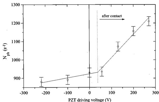
FIG. 3. Dependence of the acceptor's fluorescence signal on the acting force recorded during the SNOM-based FRET experiment. The contact point was determined from the change in oscillation amplitude of the tip.
