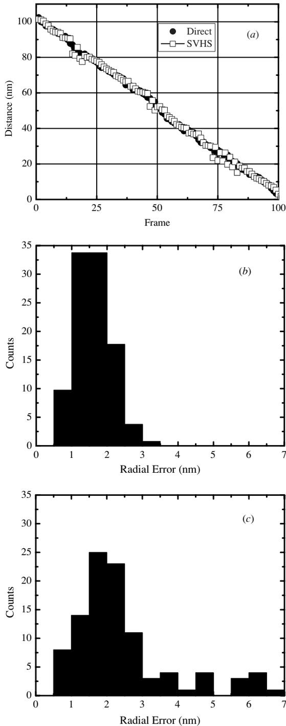
**Figure 4.** Effects of cassette tapes on tracking accuracy. (a) Tracking from SVHS video tapes reduces the accuracy by about 0.5 nm with respect to direct tracking from a 30 nm/pixel camera, resulting in a more noisy track. In the distribution of radial errors for direct tracking (b) and SVHS tracking (c) a longer tail is observed for tracking done from SVHS. SVHS appears smoother than VHS in general (data not shown).
