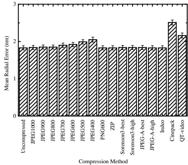
**Figure 5.** The accuracy of the tracking method for different image compression formats. Only Cinepack showed a large change compared to the uncompressed result. All other stacks were generated by compressing/decompressing the stack used to obtain the results for the 'unknown' column. The image stack was made from a data set at 33 nm/pixel, S/N of 13.9. Error bars represent SEM for 550 measurements.
