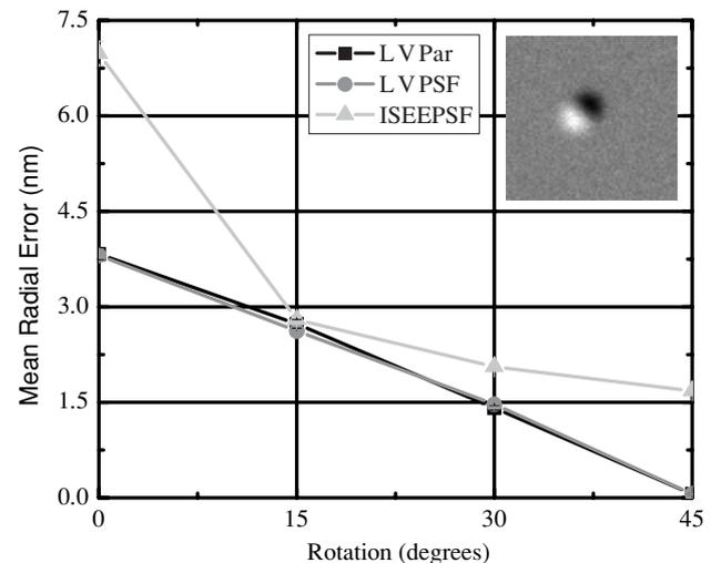
**Figure 6.** Rotation of DIC image versus mean radial error for the parabolic methods. Notice how the error falls almost linearly with rotation aligning the axis of symmetry with the  $x$  axis. Error bars represent the SEM and are smaller than the symbols. The inset shows an un-rotated simulated DIC image of a bead.
