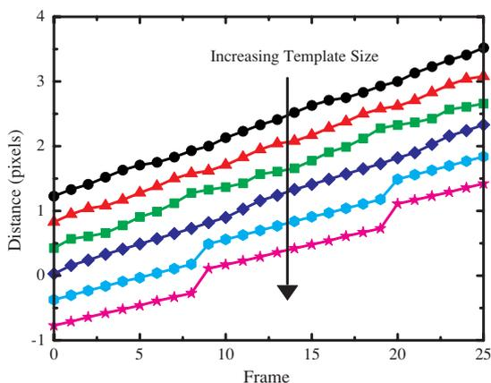
**Figure 10.** ISee-CM tracks at different template sizes (tracks offset for clarity). Note that at larger sizes a non-existent step is observed. These results are for a no-noise image stack. Template size, from top to bottom: 22, 26, 30, 40, 50, 60 pixels.
