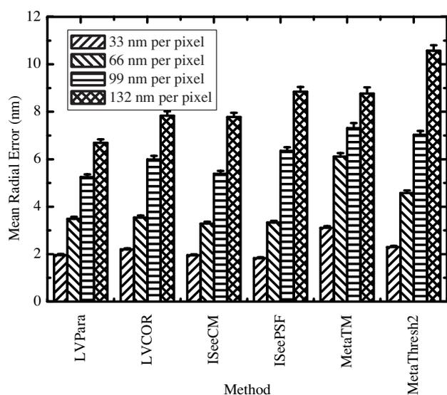
**Figure 11.** Mean radial error versus magnification for different tracking methods. The mean radial error scales with magnification. On average, four times more magnification means four times more accuracy. Error bars represent SEM for 550 measurements.
