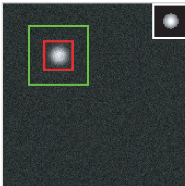
**Figure 1.** A sample image used during testing of the different tracking algorithms. The inner square is the template chosen, the outer square is the search area. Inset: a sample correlation image taken during execution of the LabVIEW COR (LVCOR) tracking algorithm. The template size is  $26 \times 26$  pixels and the search region is  $54 \times 54$  pixels which results in a square correlation image with  $(54-26) + 1$  pixels on each side.
