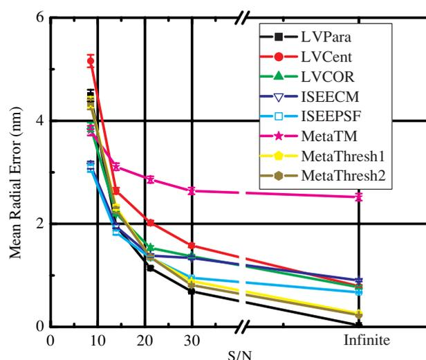
**Figure 2.** The accuracy of the different tracking methods as a function of S/N. MetaThresh1 and 2 do the best from S/N 29.9 to S/N 13.9. At S/N 8.5 the ISee methods achieve the best results, while the accuracy of LabVIEW Cent falls to an unacceptable level. The magnification was 33 nm/pixel. Error bars represent the SEM for 550 measurements.
