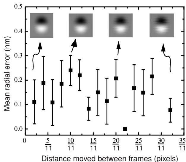
**Figure 8.** Mean radial error versus fractional pixel movement between frames. Error bars are standard deviation. Inset shows (from left to right) the appearance of the 2/11, 10/11, 20/11 and 32/11 objects.
