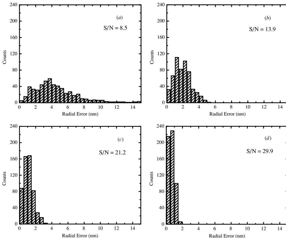
**Figure 3.** As S/N changes, so does the distribution of radial errors. At an S/N of 8.5 (a) the radial error shows the greatest spread. As S/N increases, this distribution becomes tighter (13.9 (b), 21.2 (c), 29.9 (d)) but never reaches zero (even at infinite S/N, data not shown). The standard deviation is typically half the mean value. All images had 33 nm/pixel and were tracked using LabVIEW Para. The distribution is representative of the other methods at the same S/N.
