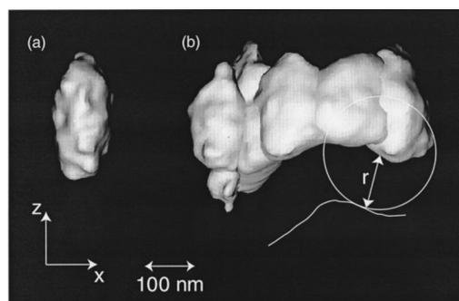
FIG. 2. Frequency isosurfaces of 5 counts per voxel of a 216 nm bead trapped by optical tweezers in solution (a) and in an agar network (b). The position of the trap was laterally scanned in the network with a stepwidth of 80 nm. The object's surface (white line) was calculated taking the radius of the bead into account (white circle). The data acquisition time at each position was 0.8 s.
