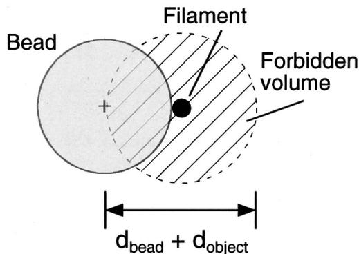
FIG. 4. Mechanical amplification effect. An mechanical stiff filamentous object with a diameter  $d_{\text{object}}$  will appear in a thermal noise scan as a cylinder with a minimal diameter of  $d_{\text{min}} = d_{\text{bead}} + d_{\text{object}}$ .
