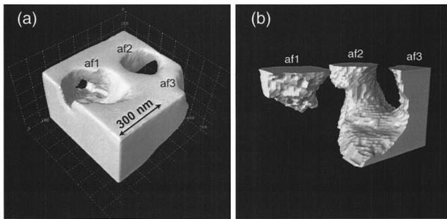
FIG. 3. 3D thermal noise image of an agar network. The volume accessible to the bead fluctuations is within the frequency isosurface (a). Volumes elements which are not accessible because of the presence of agar filaments appear either as channels (af1 and af2) or as additional constraint of the overall volume (af3). The inverse image (b) represents the volume not accessible to the bead.
