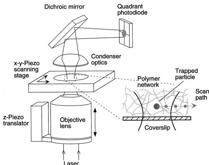
FIG. 1. Experimental setup and procedure. To image a part of an agar network, a 216 nm latex bead is trapped by optical tweezers at low laser power and then scanned stepwise through the network. The dots on the scan path indicate the different energy minimum position of the optical trap around which the bead fluctuates and probes its local environment.
