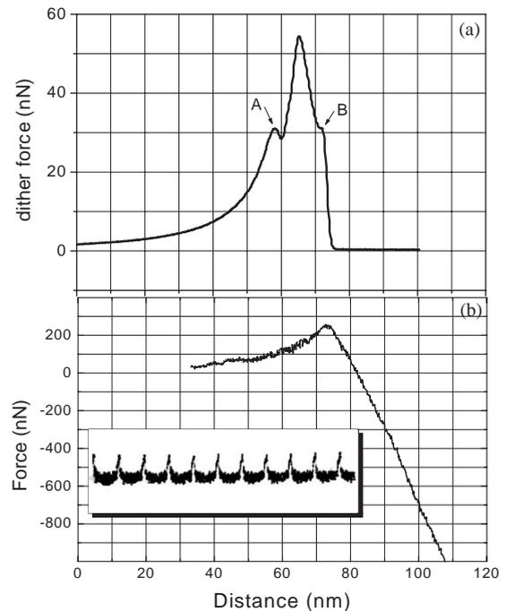
Fig. 2. Approach curves for the dithering force (a) and corresponding cantilever deflection (calibrated in force units), (b) for the resonantly driven probe ( $f = 13.8$  kHz,  $Q \sim 800$ ). Dither amplitude—30 nm. In the inset the oscilloscope trace of the AFM cantilever deflection shows peaks due to tapping at the dither frequency of fiber tip.
