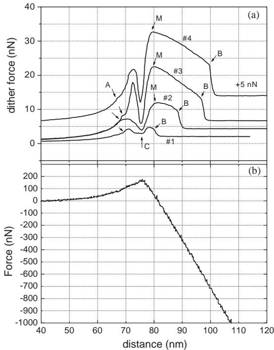
Fig. 4. Approach dither force and static force curves for the non-resonantly driven probe ( $f = 8$  kHz), optical detection. Dither amplitude: #1—4 nm, #2—9 nm, #3—14 nm, #4—18.5 nm.
