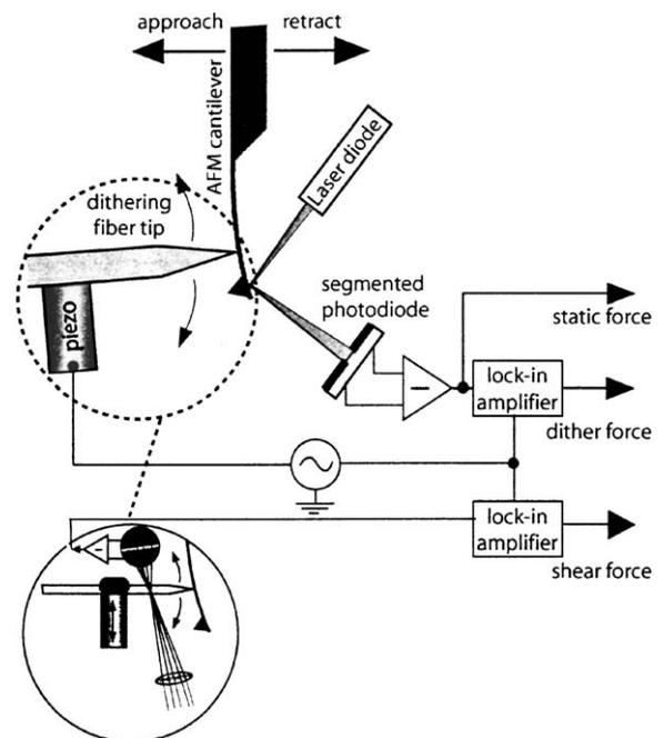
Fig. 1. Schematic diagram of the experimental setup (not to scale). The fiber tip is positioned over the flat portion of the AFM cantilever. The interaction force is measured via the deflection of cantilever. In the inset the optical method of dither amplitude control is shown.
