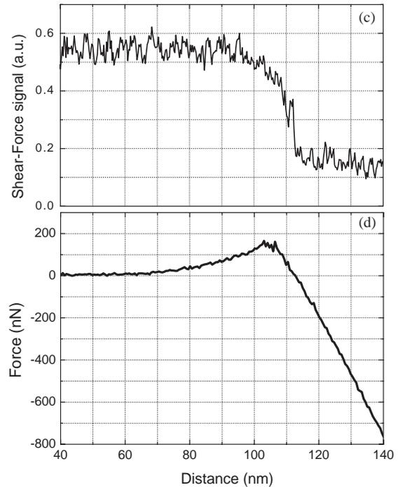
Fig. 3. Approach curves for the shear force signal (c) and corresponding cantilever deflection (calibrated in force units), (d) for the non-resonantly driven probe ( $f = 8$  kHz). Dither amplitude—4 nm.
