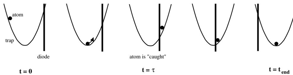
**Figure 2.** Schematic representation of the cooling method for a single particle: snapshots for different times; the passing direction of the diode is from left to right.
