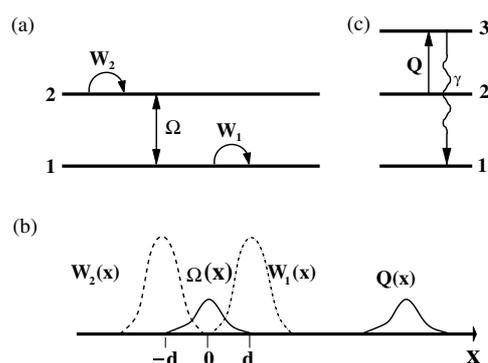
**Figure 1.** (a) Schematic action of the different lasers on the atom levels; (b) location of the laser potentials; (c) schematic action of a quenching laser.
